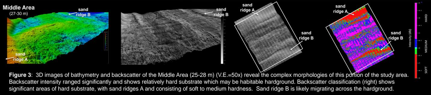
**Figure 3:** 3D images of bathymetry and backscatter of the Middle Area (25-28 m) (V.E.=50x) reveal the complex morphologies of this portion of the study area. Backscatter intensity ranged significantly and shows relatively hard substrate which may be habitable hardground. Backscatter classification (right) shows significant areas of hard substrate, with sand ridges A and consisting of soft to medium hardness. Sand ridge B is likely migrating across the hardground.
